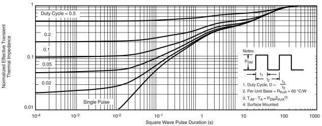
Normalized Thermal Transient Impedance, Junction-to-Ambient
