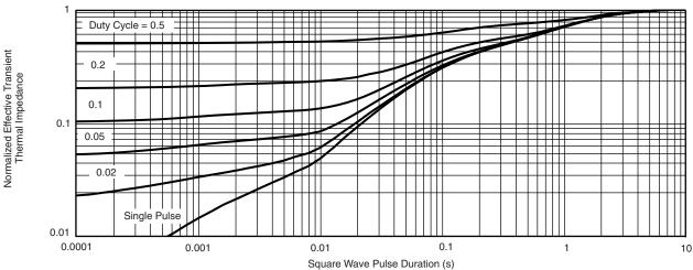
Normalized Thermal Transient Impedance, Junction-to-Foot
