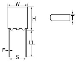
Series T340 Dielectric MnO2 Tantalum Style Radial Molded Radial, Solid Tantalum, Molded Description RoHS Yes Termination Tin AEC-Q200 No Construction Molded Includes Standoff Height of 0.38 +/- 0.13mm. Miscellaneous Longest Lead Is Positive. Notes
