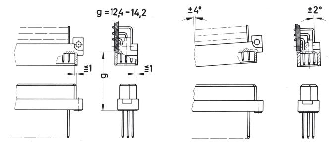
To ensure reliable connections and prevent unnecessary damage, please refer to the application data diagrams. These recommendations are set out in IEC 60603-2.
