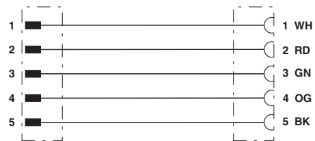
Contact assignment of 7/8" plug
