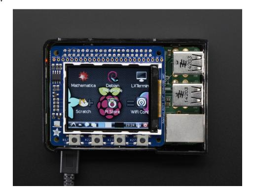
The cute PiTFT got even more adorable with this little primary display for Raspberry Pi in HAT form! It features a 2.2" display with 320x240 16-bit color pixels. The HAT uses the high speed SPI interface on the Pi and can use the mini display as a console, X window port, displaying images or video etc. Best of all it plugs right in on top of your Model A+ or B+ and fits into our case quite nicely.
