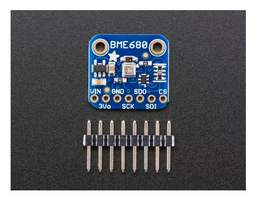
For your convenience we've pick-and-placed the sensor on a PCB with a 3.3V regulator and some level shifting so it can be easily used with your favorite 3.3V or 5V microcontroller.
