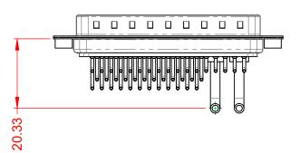
20A (CURRENT) POWER/CO-AX CONTACT RATING: (IF PRESENT) SIGNAL CONTACT CURRENT RATING: 5A PER CONTACT SIGNAL CONTACT RESISTANCE:  $10m\Omega$  MAX. **INSULATOR RESISTANCE:** 5000MΩ min. DIELECTRIC
