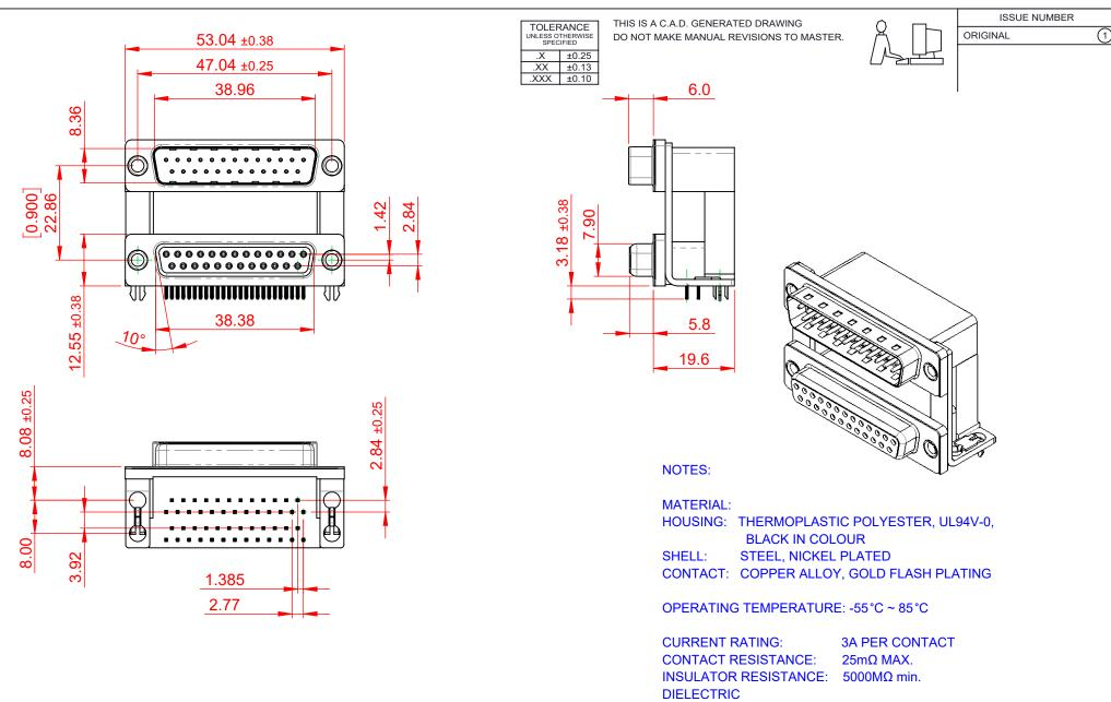
WITHSTANDING VOLTAGE: 1000V AC rms
