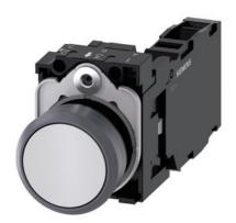
Pushbutton, 22 mm, round, plastic with metal front ring, white, pushbutton, flat, momentary contact type, with holder, 1 NO+1 NC, screw terminal, with laser labeling, inscription or symbol Customer-specific selection with SIRIUS ACT configurator (CIN)
