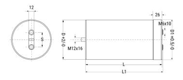
General Information Series C44U-M Dielectric Metallized Polypropylene Style DC Filtering, Energy Storage Features RoHS With Exemptions **REACH** SVHC (Pb - CAS 7439-92-1) SCIP Number cc1c1ec4-db9e-4815-b26b-e8a34ddfb776 Screw Terminals M6 Lead AEC-Q200 Nο Component 960 g Weight Thermal Resistance = 6.4 C/W. Weight = 4800 Miscellaneous grams.
