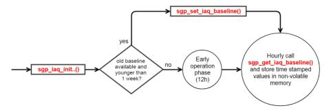
Call sgp\_iaq\_init\_continuous () to reset all SGP baselines. After the accelerated warm-up phase (see 3.9. for durations), the initialization takes 20 seconds, during which the IAQ output will not change.
