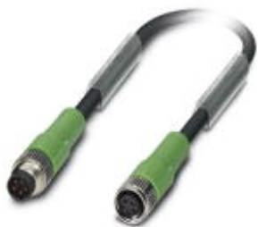
Sensor/actuator cable, 5-position, PUR halogen-free, black-gray RAL 7021, Plug straight M8, B-coded, on Socket straight M8, B-coded, cable length: 1.5 m
