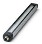
LED machine light, 24 V DC, emission angle 85 °/95 °, color temperature 5000 K, length 365 mm, diameter 40 mm, M12 connector, Light housing: Anodized aluminum, Pane: Single-pane safety glass (ESG, thermally toughened float glass), pivoting, resistant to coolants and lubricants, can be switched in series
