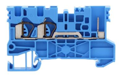
Feed-through terminal, Tension-spring connection, Mounting type: Mounting rail TS 35/7.5, Rated cross-section: 2.5 mm², Width: 5.1 mm, Colour: Blue
