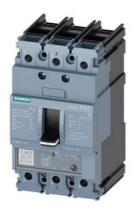
circuit breaker 3VA5 UL frame 125 breaking capacity class M 35kA @ 480 V 3-pole, line protection TM230, FTAM, In=70A overload protection Ir=70A fixed short-circuit protection li=5...10 x In cable connection on both sides
