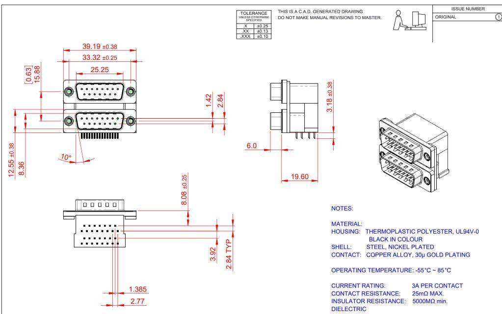
WITHSTANDING VOLTAGE: 1000V AC rms
