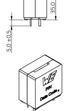
Pin 2 and 3 are only for mechanical stability.
