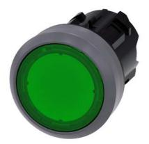
Indicator light in illuminated pushbutton design, 22 mm, round, plastic with metal front ring, green, with laser labeling, upper case and lower case, always upper case at beginning of line
