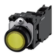
Illuminated pushbutton, 22 mm, round, plastic, yellow, pushbutton, flat, momentary contact type, with holder, 1 NO+1 NC, LED module with integrated LED 24 V AC/DC, spring-type terminal, with laser labeling, upper case
