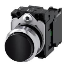
Pushbutton, 22 mm, round, metal, shiny, black, pushbutton, raised, momentary contact type, with holder, 1 NO, screw terminal, with laser labeling, symbol number according to, ISO 7000 or IEC 60417
