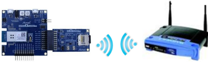
Figure 4-31. The SAM W25 Xplained Pro and the IO1 Xplained Pro Header (for MicroSD Storage)
