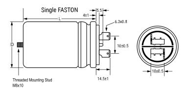
General Information Series C87 Dielectric Film/Foil Polypropylene Style Aluminum Case, Plastic Cover, Spun Seal Description Features Spun Seal, Safety Class S2, UL\_94 V0 Disk RoHS Yes Lead Fast On (1+1) UL, VDE, CQC, CSA (600VAC), UL\_94 V0 Qualifications Disk AEC-Q200 No Component 79 g Weight
