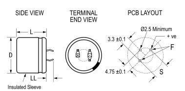
**General Information** Series PEH526 Dielectric Aluminum Electrolytic Description Snap-In, Aluminum Electrolytic RoHS Lead 3 Pin Short Qualifications AEC-Q200 AEC-Q200 Yes Component Weight 14 g Notes Add 0.5mm To D And 1mm To L For Sleeving. Shelf Life 520 Weeks
