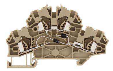
Double-level terminal with electronic components, Tension-spring connection, Mounting type: Mounting rail TS 35/7.5, Rated cross-section: 2.5 mm<sup>2</sup>, Width: 5.1 mm, Colour: Beige
