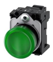
Indicator lights, 22 mm, round, plastic, green, lens, smooth, with holder, LED module, with integrated LED 24 V AC/DC, spring-type terminal, with laser labeling, symbol number according to, ISO 7000 or IEC 60417
