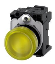
Indicator lights, 22 mm, round, Metal, shiny, yellow, lens, smooth, with holder, LED module with integrated LED 230 V AC, spring-type terminal, with laser labeling, symbol number according to, ISO 7000 or IEC 60417
