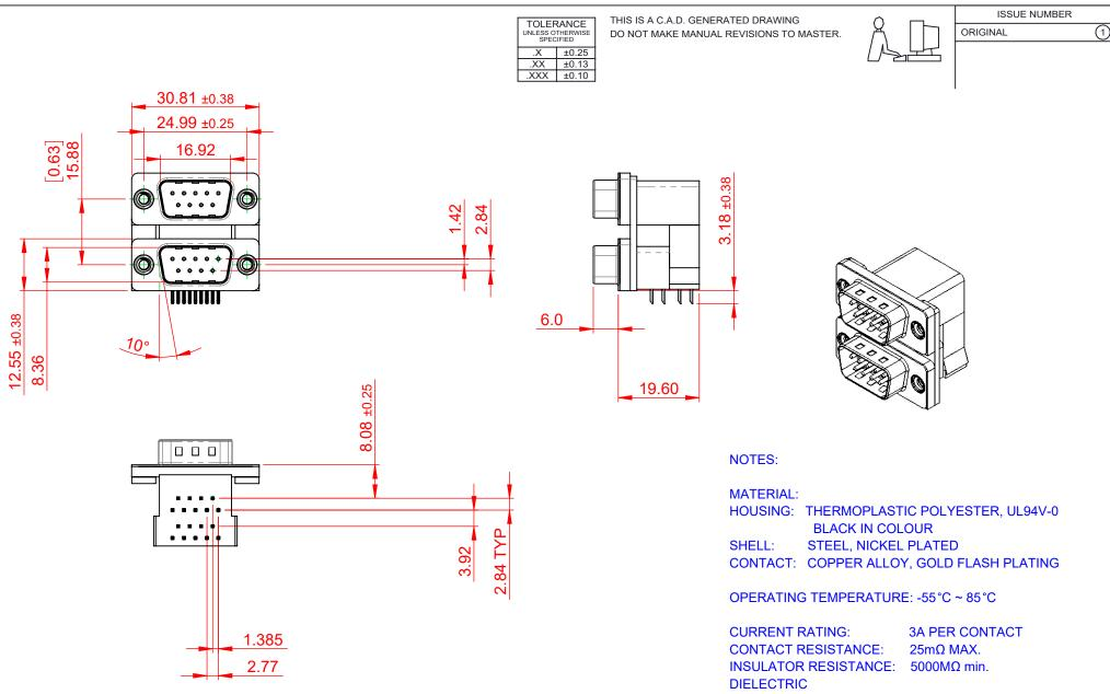
WITHSTANDING VOLTAGE: 1000V AC rms
