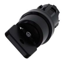
Key-operated switch O.M.R, 22 mm, round, plastic, lock number 73034, black, with 2 keys, 2 switch positions O<I, momentary contact type, Actuating angle 45°, 10:30h/12h, key removal O, with laser labeling, upper case
