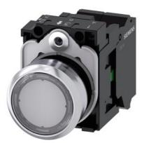
Illuminated pushbutton, 22 mm, round, metal, shiny, clear, pushbutton, flat, momentary contact type, with holder, 1NO, LED module with integrated LED 110 V AC, spring-type terminal, with laser labeling, upper case
