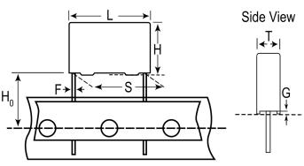
Style Radial Features MKP EMI Safety RoHS Lead Wire Leads Safety Class X1 Qualifications ENEC, UL, cUL, CQC AEC-Q200 No THB Performance No 2.013 g Component Weight Miscellaneous ClimCat: 40/110/56/C. Shelf Life 104 Weeks
