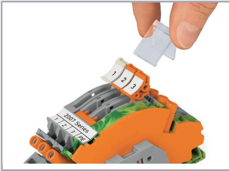
Using locking covers or profiles for adjacent terminal blocks allows disconnect links to be operated simultaneously.
