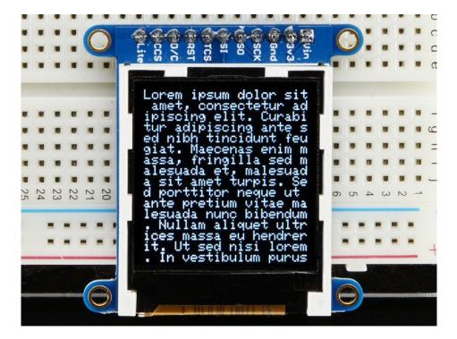
The 1.44" display has 128x128 color pixels. Unlike the low cost "Nokia 6110" and similar LCD displays, which are CSTN type and thus have poor color and slow refresh, this display is a true TFT! The TFT driver (ST7735R) can display full 16bit color using our library code.
