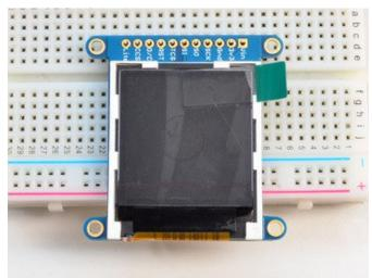
Add the breakout board: Place the breakout board over the pins so that the short pins poke through the breakout pads
