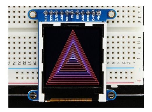
The breakout has the TFT display soldered on (it uses a delicate flex-circuit connector) as well as a ultra-low-dropout 3.3V regulator and a 3/5V level shifter so you can use it with 3.3V or 5V power and logic. We also had a little space so we placed a microSD card holder so you can easily load full color bitmaps from a FAT16/FAT32 formatted microSD card. The microSD card is not included, but you can pick one up here (http://adafru.it/102).
