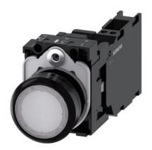
Illuminated pushbutton, 22 mm, round, plastic, white, pushbutton, flat, momentary contact type, with holder, 1 NO+1 NC, LED module with integrated LED 24 V AC/DC, spring-type terminal, with laser labeling, symbol number according to, ISO 7000 or IEC 60417
