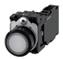
Illuminated pushbutton, 22 mm, round, plastic, clear, pushbutton, flat, momentary contact type, with holder, 1 NO+1 NC, LED module with integrated LED 110 V AC, screw terminal, with laser labeling, upper case
