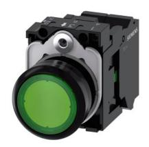
Illuminated pushbutton, 22 mm, round, plastic, green, pushbutton, flat, momentary contact type, with holder, 1NO, LED module with integrated LED 230 V AC, spring-type terminal, with laser labeling, lower case
