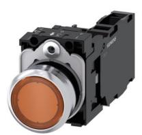
Illuminated pushbutton, 22 mm, round, metal, shiny, amber, pushbutton, flat, momentary contact type, with holder, 1 NO+1 NC, LED module with integrated LED 24 V AC/DC, screw terminal, with laser labeling, upper case
