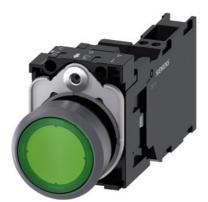
Illuminated pushbutton, 22 mm, round, plastic with metal front ring, green, pushbutton, flat, momentary contact type, with holder, 1 NO+1 NC, LED module with integrated LED 24 V AC/DC, spring-type terminal, with laser labeling, symbol number according to, ISO 7000 or IEC 60417
