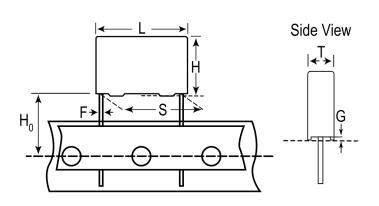
Series F881 Dielectric Metallized Polypropylene Style Radial Features MKP EMI Safety RoHS Lead Wire Leads Safety Class Qualifications ENEC, UL, cUL, CQC AEC-Q200 No THB Performance No 0.876 g Component Weight Miscellaneous ClimCat: 40/110/56/C. Shelf Life 104 Weeks
