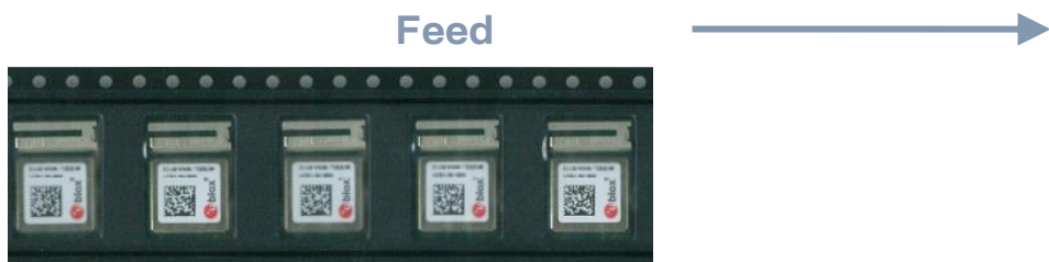
Figure 11: Orientation of NINA-B222 module on tape
