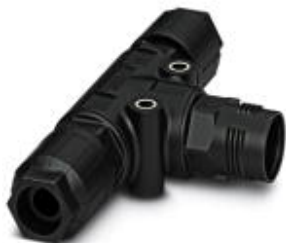
T distributor, QUICKON connection, number of positions: 4+PE, 0.5 mm 2 ... 1.5 mm 2 , 690 V, 17.5 A, black, With two QUICKON nuts, cable diameter range: 5 mm ... 10 mm
