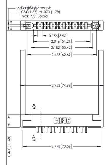
A-A0.295[7.49] Card Slot **ECTION** 0.090[2.29] Point of Contact 305 ENG MASTER 305 / 315 / 355 Card Edge Connector
