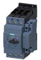
Circuit breaker size S2 for motor protection, CLASS 10 with overload relay function A-release 12...17 A N-release 260 A Standard switching capacity
