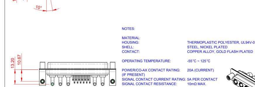
SW REFERENCE NO .: 630 COMBO ASSEMBLY COMBINATION D-SUB DRAWN: C.B DATE: JAN. 01/2019 CHECKED: DATE: THESE DRAWINGS AND SPECIFICATIONS SCALE: (IN C.A.D. 1:1) SHEET 1 DAC INC ARE THE PROPERTY OF EDAC INC..AND 630-17W5240-2ND DRAWING NUMBER:
