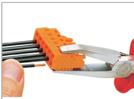
Inserting a conductor via operating tool.
