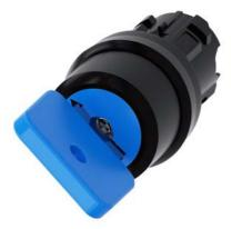
Key-operated switch O.M.R, 22 mm, round, plastic, lock number 73038, blue, with 2 keys, 2 switch positions O<I, momentary contact type, Actuating angle 45°, 10:30h/12h, key removal O, with laser labeling, upper case
