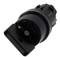
Key-operated switch O.M.R, 22 mm, round, plastic, lock number 73034, black, with 2 keys, 2 switch positions O<I, momentary contact type, Actuating angle 45°, 10:30h/12h, key removal O, with laser labeling, inscription or symbol Customer-specific selection with SIRIUS ACT configurator (CIN)
