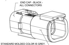
4 POS, RECEPTACLE, PIN, ATM SERIES, SNAP FIT
