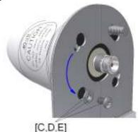
Repeat for remaining screws x2. Assemble (AWG-6/16mm^2 min) Grounding cable to crimp lug [J] fasten with supplied hardware [F,G,H]. Do not over tighten - Recommended torque 5-8lbf\*in [1Nm.
