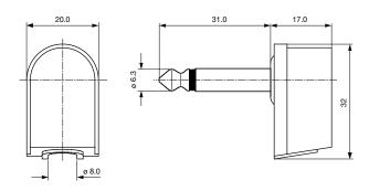
Cable diameter max. 8.0 mm
