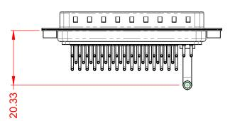
POWER/CO-AX CONTACT RATING: 30A (CURRENT) (IF PRESENT) SIGNAL CONTACT CURRENT RATING: 5A PER CONTACT SIGNAL CONTACT RESISTANCE:  $10m\Omega$  MAX. INSULATOR RESISTANCE:  $5000M\Omega$  min. DIELECTRIC
